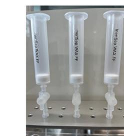
Fig.3 Solid Phase Extraction Procedure for PFAS Recovery Test in Tap Water
